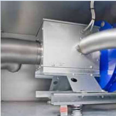
encapsulated motor with separate ventilation
